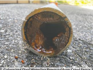
Galvanized Steel Waterline Removed from Crawl Space
